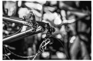
Fasten the dérailleur to the hanger, ensuring that they are aligned correctly (with b-tension screw in contact with the dérailleur's plastic washer rather than the hanger).
