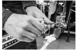
Bolt the front brake caliper to the fork's lower leg. This must be centered with the brake rotor once the wheel is installed.
